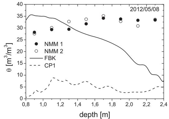
Fig. 5 Comparison of spatial soil moisture profiles of NMM measurements and reconstructed UWB measurement.
