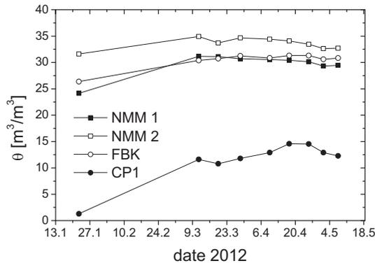
**Fig. 6 Comparison of NMM and spatial TDR measurements of volumetric water content  $\theta$  and data from first two quarters of year 2012 at a depth of 130 cm.**
