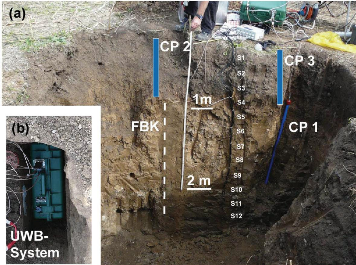
Fig. 3 Overview of the measurement location (a) installed sensors (CP 1, FBK and S 1 -12 as well as location of the sensors CP 2 and 3 after filling up the hole) and (b) measurement system after instrumentation of the measurement site.
