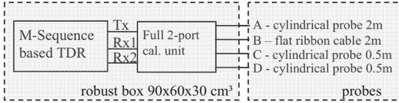
Fig. 1 Block diagram of TDR Measurement System.
