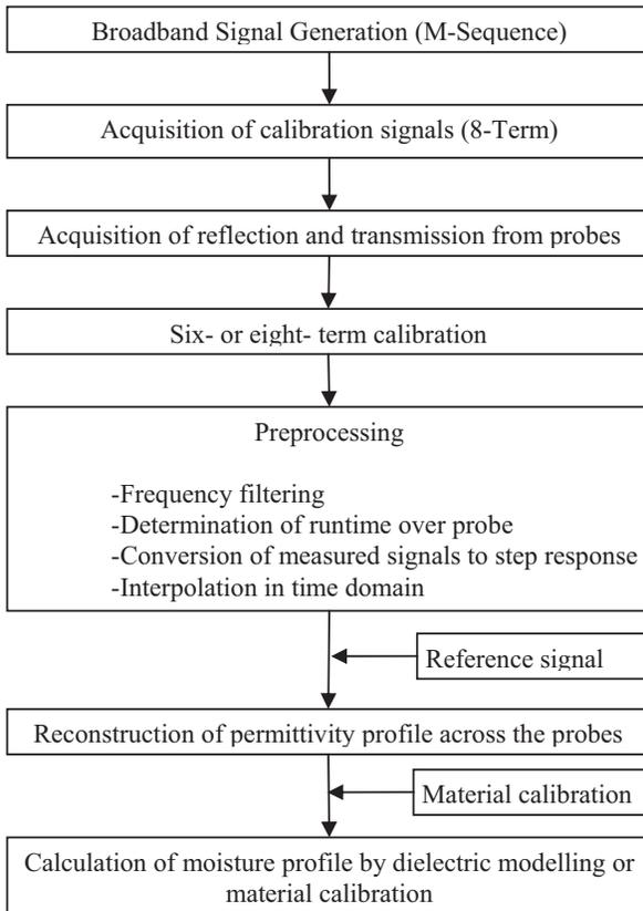
Fig. 2 Schematic of measurement cycle.
