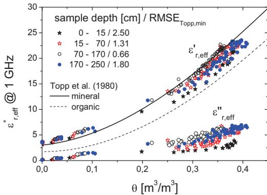
Fig. 4 Relationship between volumetric water content  $\theta$  and relative effective permittivity  $\epsilon_{r,eff}^* = \epsilon'_{r,eff} - j\epsilon''_{r,eff}$  at a frequency of 1 GHz obtained with the methodology according to Lauer et al. (2012) [9] and Wagner & Lauer (2012) [10].
