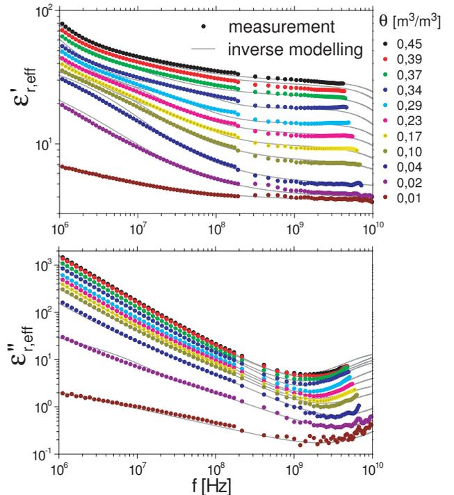
Fig. 1. Real part  $\varepsilon'_{r,\text{eff}}$  and imaginary part  $\varepsilon''_{r,\text{eff}}$  of the experimental determined complex relative effective permittivity  $\varepsilon^*_{r,\text{eff}}$  as a function of frequency for different volumetric water contents  $\theta$ .
